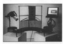
The Timetrack 25 lens curved close-up camera is configured in a 130-degree arc spanning 21" inches with an eight-inch radius and lenses that focus and converge at eight inches. It shoots
